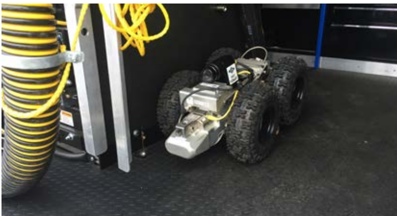
Camera used for pipe assessments
